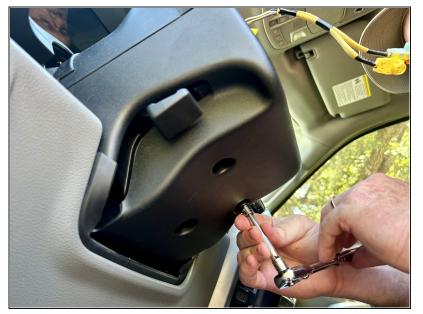
Move the steering column covers back into place and replace the three screws underneath using a socket wrench and 7mm socket.
