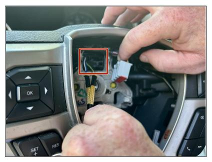
Unclip and disconnect the steering wheel wires at the top.
