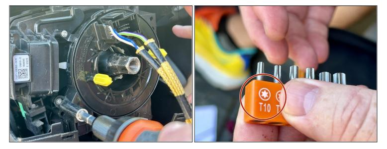
• Unscrew the broken clockspring using a Torx screwdriver and T10 bit to remove the four screws holding it in place.
