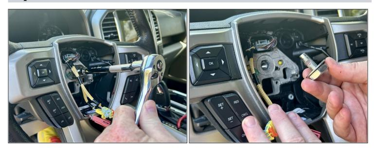
• Use a socket wrench and 24mm socket to remove the steering wheel bolt.
