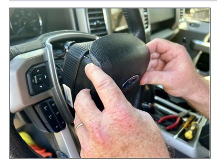
Return the airbag to its place and push it to clip it back in place.
