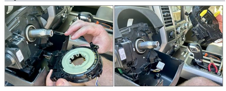
• Remove the broken clockspring and set it aside.
