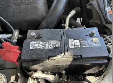
• Disconnect the cables to your vehicle battery using a socket wrench and 10mm socket.
