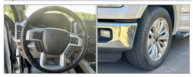
• Make sure that your steering wheel and wheels are in the straight position.
