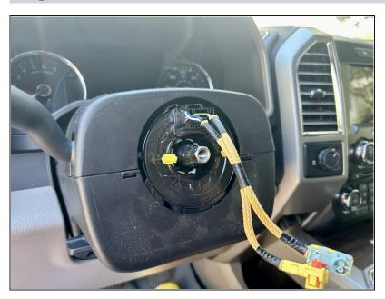
Pull the steering wheel away from the steering column and set aside.
